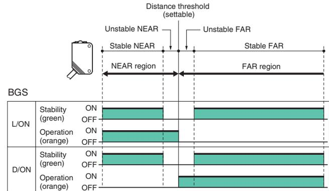
Note: If the stability indicator is lit, the detection/no detection status is stable within the rated ambient operating temperature (-10 to 55°C).
