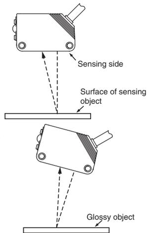
If the sensing object has a glossy surface, however, incline the Sensor by 5° to 10° as shown in the illustration, provided that the Sensor is not influenced by background objects.
