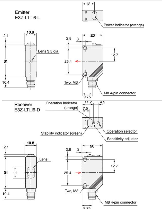
\* Model numbers for Through-beam Sensors (E3Z-LT□□) are for sets that include both the Emitter and Receiver. The model number of the Emitter is expressed by **Tel. 3103-2100 / zycon@zycon.com.br**, the model number of the Receiver, by adding "-D" (example: E3Z-LT61-D 2M). Refer to Ordering Information to modify model number of Emitters and Receivers. <http://www.zycon.com.br>
